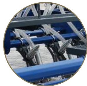
Spring tines offers machine safety
