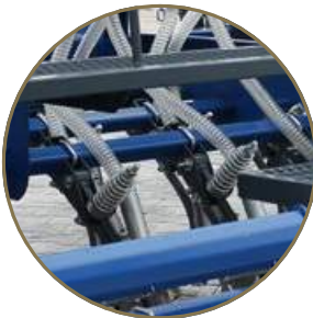
Spring tines offers machine safety
