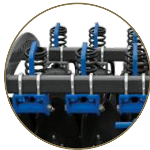
Uninterrupted tillage with independent springs
