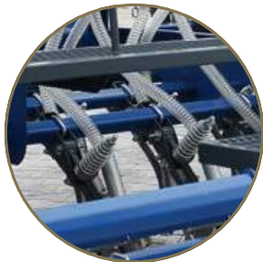
Spring tines offers machine safety
